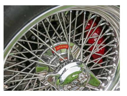
Top: the much-modified E-type looks superb in a McLaren shade of Palladian Silver grey Above: Brembo brakes hide behind 72-spoke • Turrino wheels. Stainless-steel valve is just about in shot in the bottom-left corner
