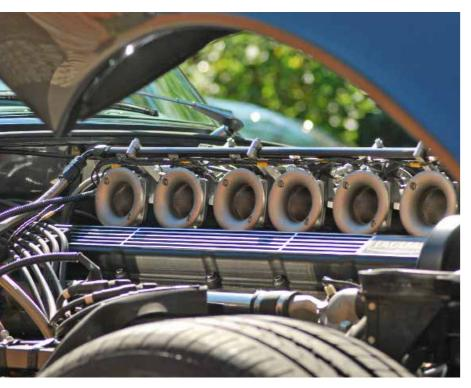
• Left and bottom: the V12 is now 6 litres, and puts out 450bhp on Jenvey throttle bodies
